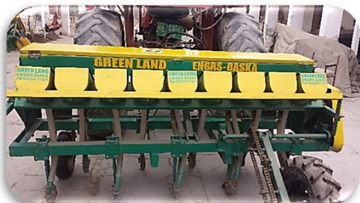
Fig. 12: Modified seed drill for DSR
