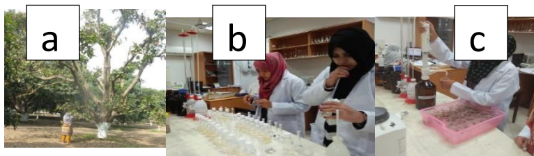
Fig. 15 shows the different steps of determination of phosphorus and potassium. a) Ammonium Acetate was used for potassium extraction of soil samples. b) The samples were filtered after centrifuging at 1500-2000 rpm for 5 minutes. c) Potassium was determined by Flame Photo Meter
