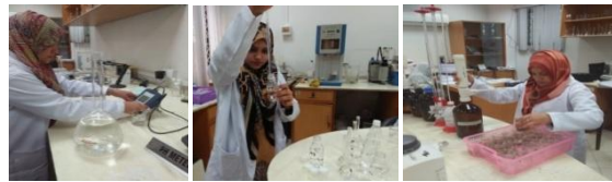
Fig. 18 \text{NaHCO}_3 preparation for soil P determination, P standards preparation, sample preparation for Soil K extraction
