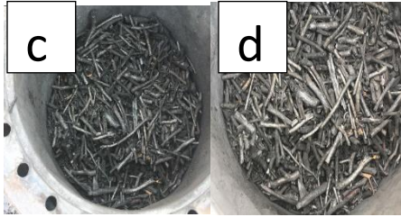
Fig. 16 the figures show the preparation of biochar on locally manufactured furnace; a) The cotton sticks and dried banana leaves were used as feed stock. The materials were grinded first before to put in furnace. b) The grinded material was put into furnace for about 45 minutes. c, d) the prepared biochar
