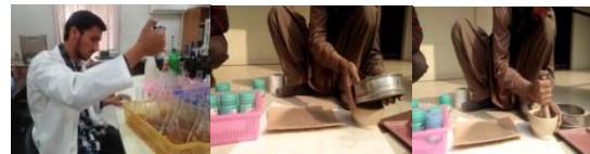
Fig. 11 Shows the different steps of organic matter determination: a) After soil samplings from the experimental field, the soils were dried for about two days. After drying, the samples were grinded, b) After grinding the samples, the soil was passed through 2mm sieve, c) Organic matter in the soil was determined by Potassium dichromate method.
