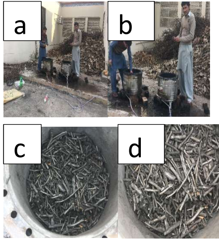
Fig. 15 The figures shows the preparation of biochar on locally manufactured furnace; a) The cotton sticks and dried banana leaves were used as feed stock. The materials were grinded first before to put in furnace. b) The grinded material was put into furnace for about 45 minutes. c, d) the prepared biochar
