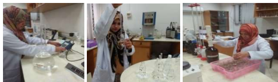
Fig. 17 NaHCO 3 preparation for soil P determination, P standards preparation, sample preparation for Soil K extraction
